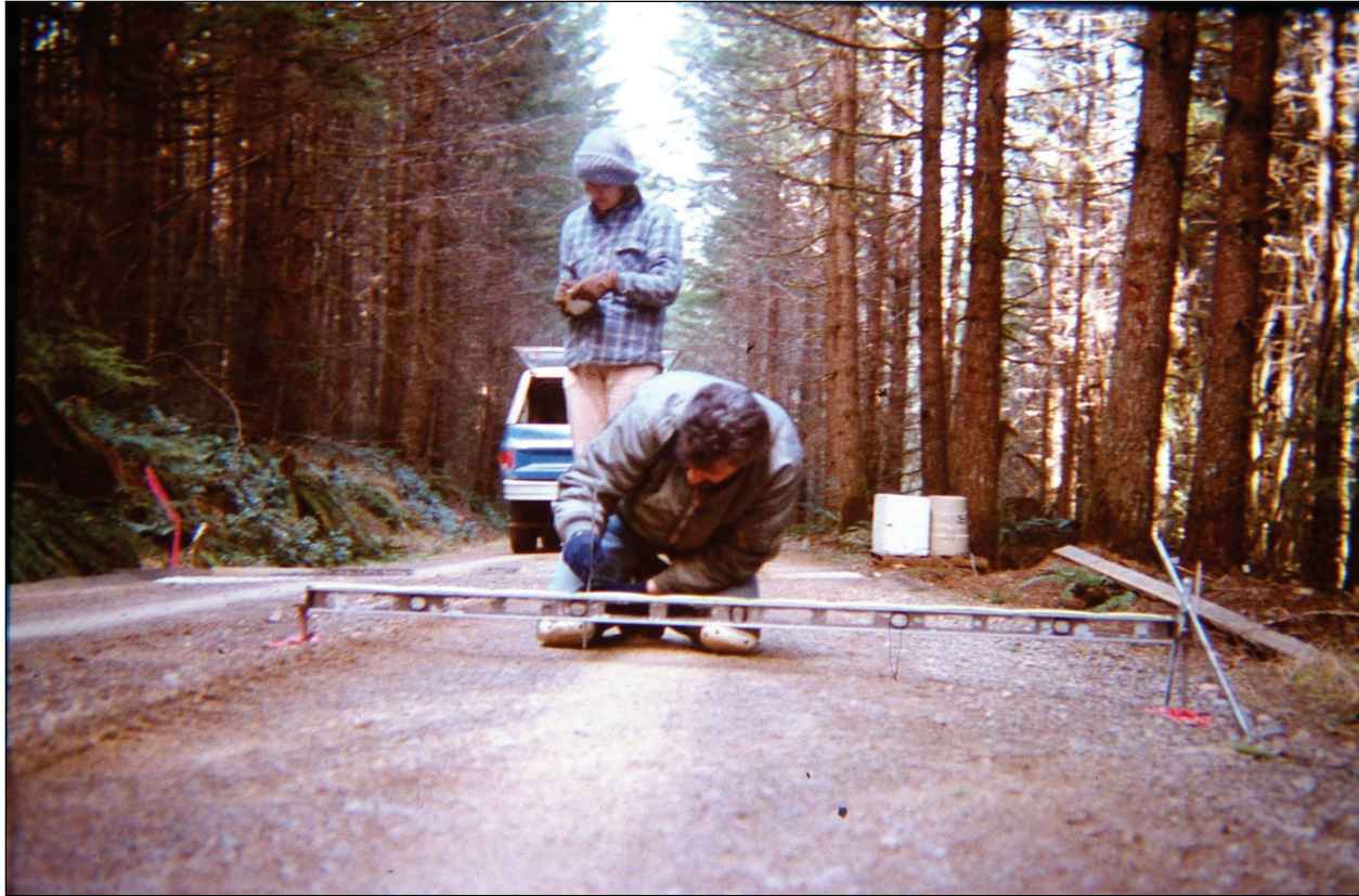
Figure 4. Measuring rut development on a logging road in the Willamette National Forest, Oregon (source: W. Elliot).
